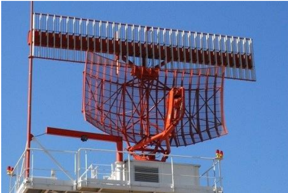
Figure 3.1 The secondary radar antenna, comprising of 35 antenna elements, on top of a STAR 2000 antenna.
