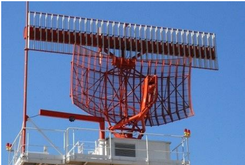
Figure 2.1 The secondary radar antenna, comprising of 35 antenna elements, on top of a STAR 2000 antenna.
