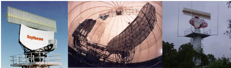
Figure 1.1: Antennas of the Raytheon ASR-10SS (left), MPR 3D radar (middle) and the Selex ATCR-33K or TAR4 (right).
