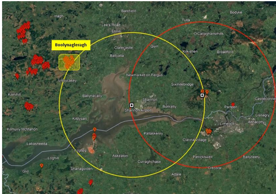
Figure 21 Boodynagleragh wind farm relative to the Eurocontrol recommended 16km assessment zone for the Shannon Airport MSSR as indicated by the yellow circle centred around the Shannon MSSR location.
