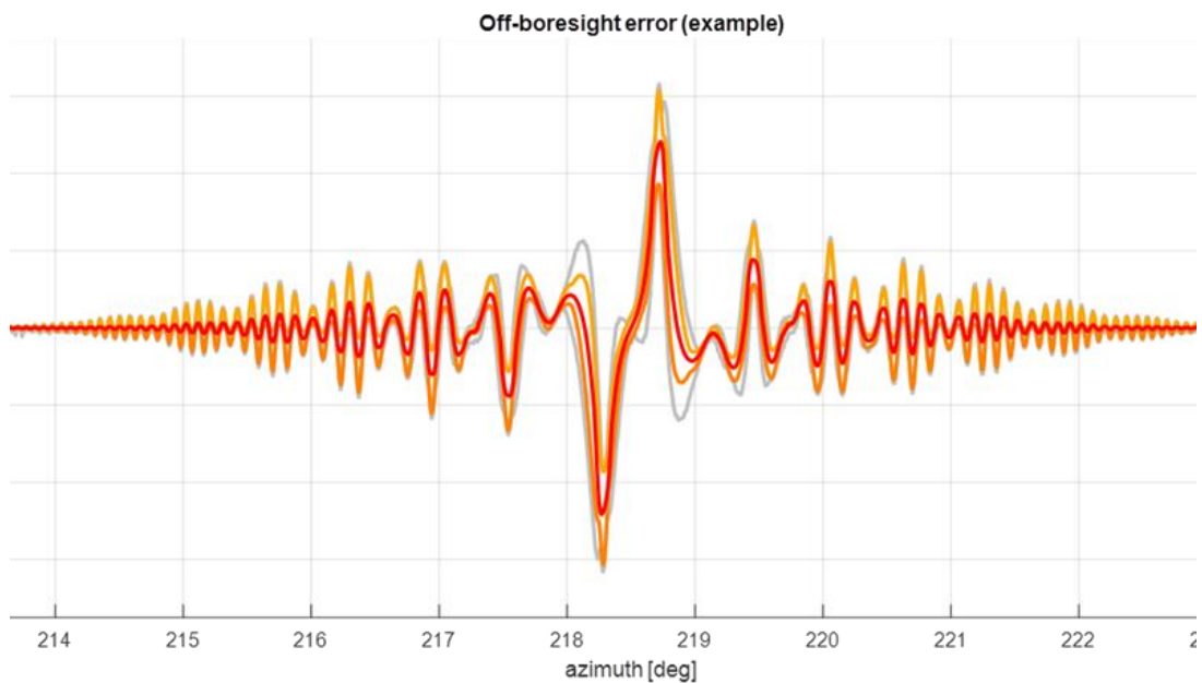
Figure 2.7 The off-boresight error for an infinite cylinder with a width of 25 m at a range of 3 km from the radar antenna. The error is point symmetrical around the azimuth angle to the obstacle.
