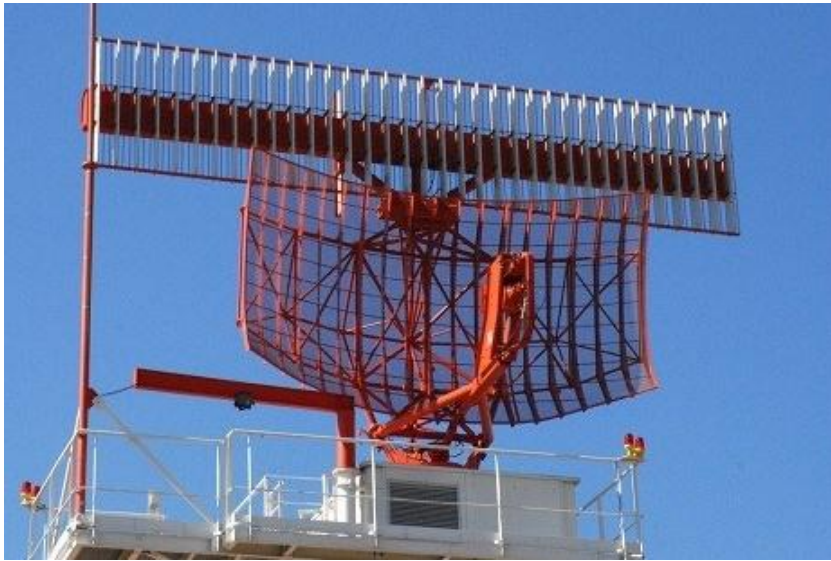
Figure 2.2 The secondary radar antenna, comprising of 35 antenna elements, on top of a STAR 2000 antenna.
