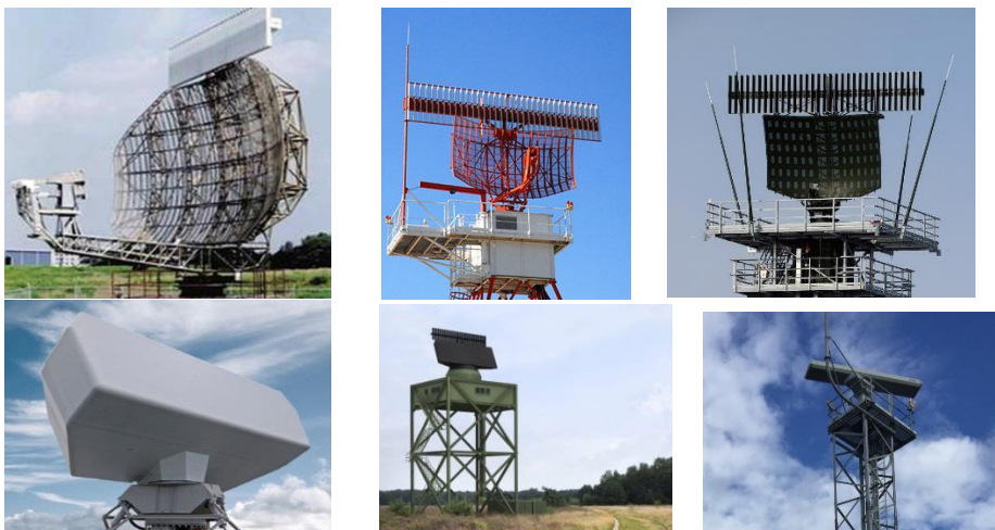
Figure 1.2: Antennas of the Raytheon ASR-23SS (top-left), Thales STAR 2000 (top-middle), Hensoldt ASR-NG (top right), Thales SMART-S Mk2 (bottom-left) and the SMART-L EWC (bottom-middle) and Terma Scanter 4002 (bottom-right).
