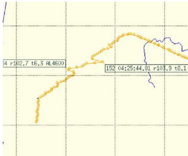
Figure 9 : Recorded ATC real track at approximately 200km as seen by the Air Traffic Controller on Radar screens
